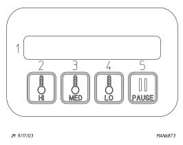
3) Verify that the applicable indicator lights on the microprocessor controller (computer) board are lit. (Refer to the **illustration below**.)
